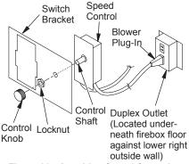
Figure 26 - Attaching Speed Control to Firebox
